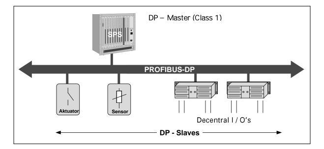
In the case of monomaster bus systems, there is only one master active at bus during the on-line phase of the bus system. The above diagram shows the system configuration of a monomaster system. The SPC based control system is the central control element. By means of the transmission medium, the DP slaves are locally linked to the SPC control system. By using this system configuration, the shortest bus cycle time can be obtained.
