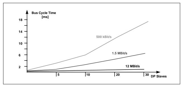
Bus cycle time of a PROFIBUS DP monomaster system Boundary conditions : Each slave has 2 byte input and 2 byte output data; the minimum slave interval time
