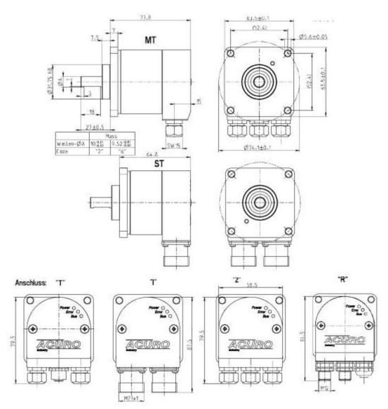
The cable screw connections require cable diameters in a range from: 7.0 ... 7.4 mm;
